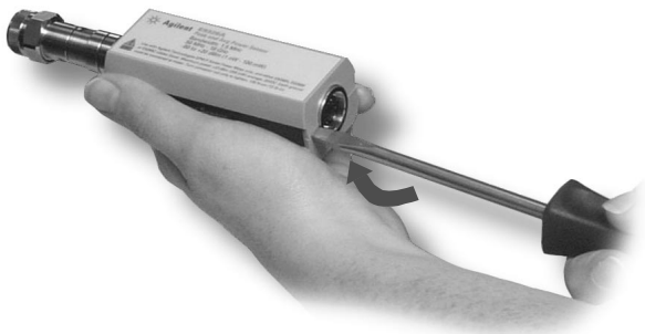
Figure 12 Removing Power Sensor Shell
